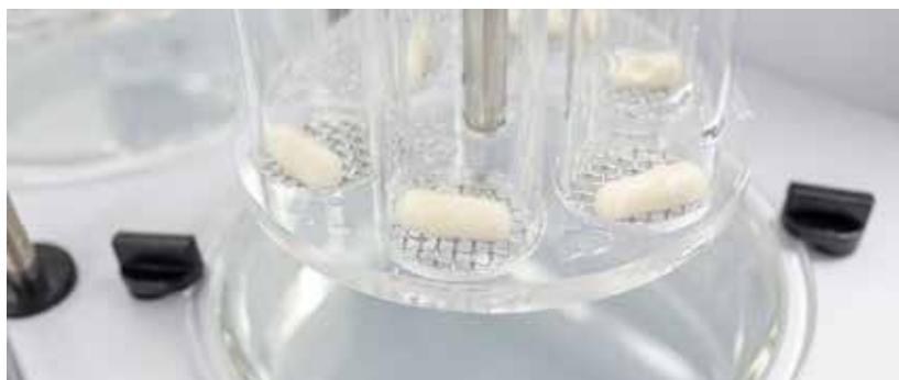
Enteric-coated capsules that resisted a simulated gastric test for 90 minutes.
